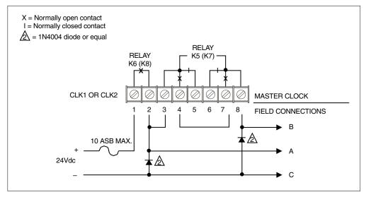
Figure B-6 Three-Wire Minute Impulse (58th Minute)
